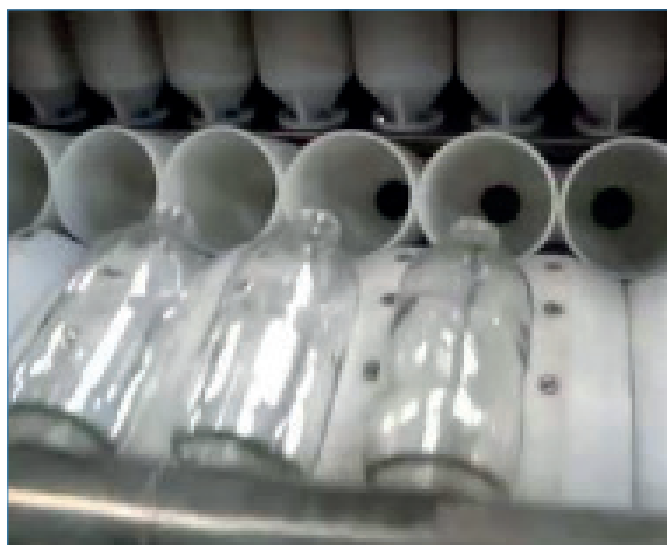
Figure 2: Loading linear washer buckets with vials
