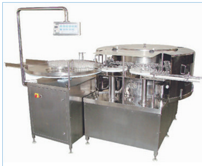
Figure 8: Rotary style washer with grippers
