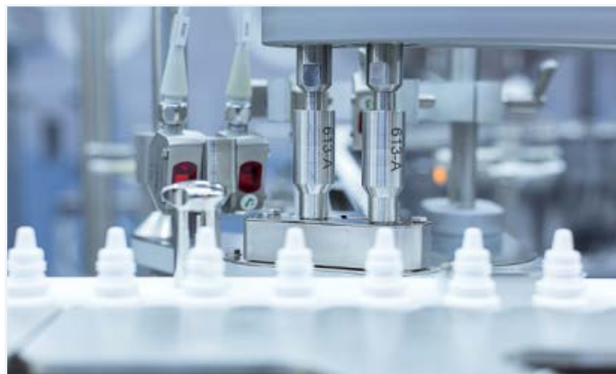
Figure 5. The two-piece eyedrop package for preservative free products is very susceptible to collapse and must be supported carefully to prevent issues
