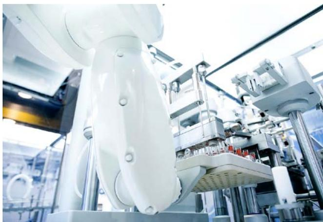
*Robot arm for cartridge filling*
