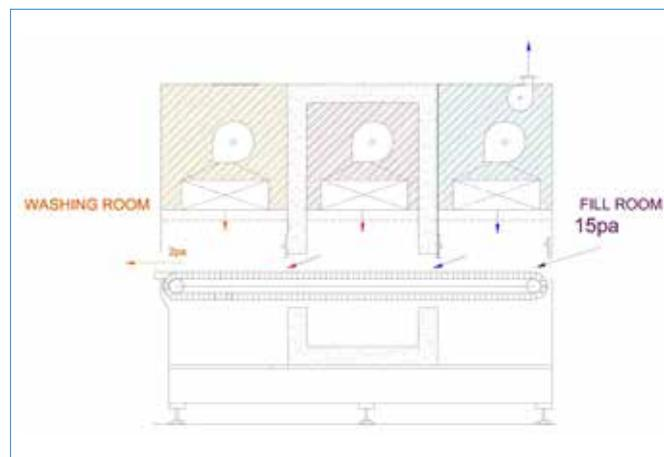
**Figure 2:** Cascading air from the Clean Room to through the hot zone. Blue Zone = cooling zone, Red Zone = Hot depyrogenation zone, Orange Zone = pre-heat zone
