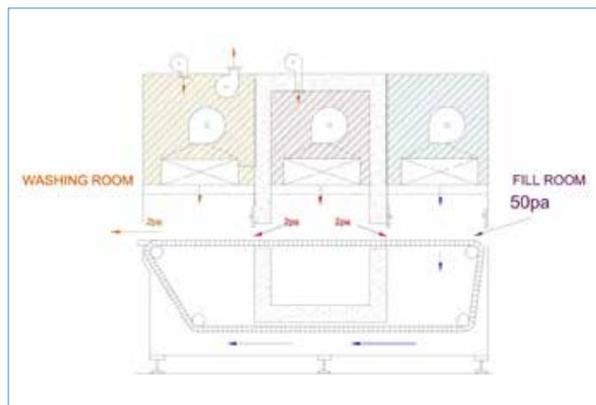
**Figure 3:** Over Pressurized Hot Zone. Blue Zone = cooling zone, Red Zone = Hot depyrogenation zone, Orange Zone = pre-heat zone
