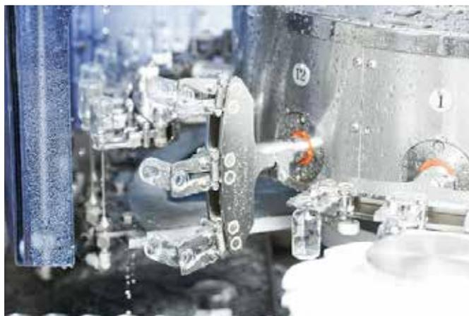
**Figure 2: Modern washing and depyrogenation installation featuring washing needles**
