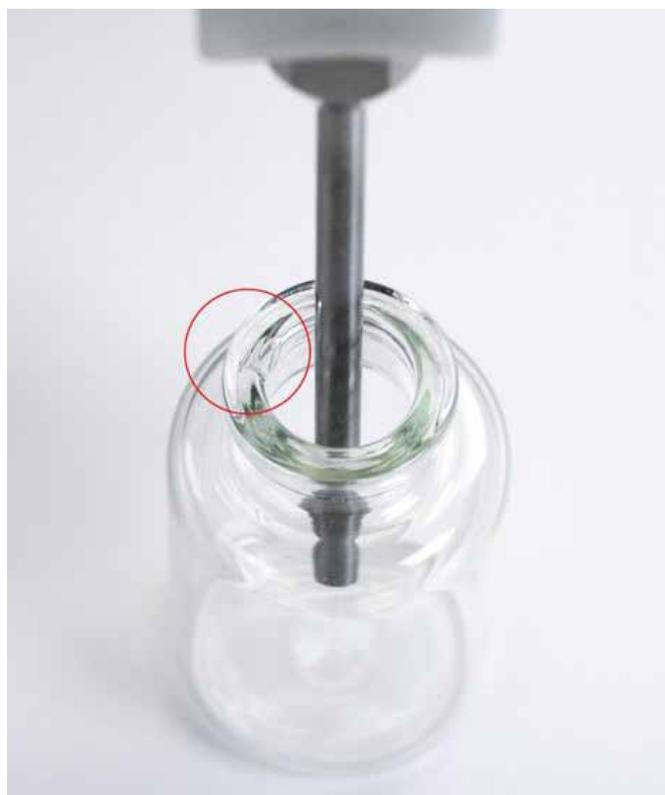
***Figure 1: Chipped vial rim and resultant particulate generation***
