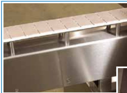
Sanitary raised-track conveyor
