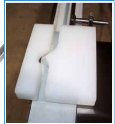
Down-vial reject blocks
