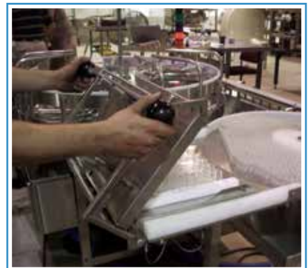
Vial inverting table
